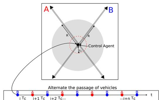
Fig. 2. Alternating principle of an intersection for two roads A and B
