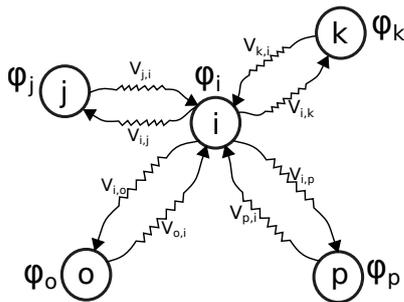
Fig. 4. The optimal phase  $\phi_i$  for intersection  $i$  depends on the phases of its neighbors
